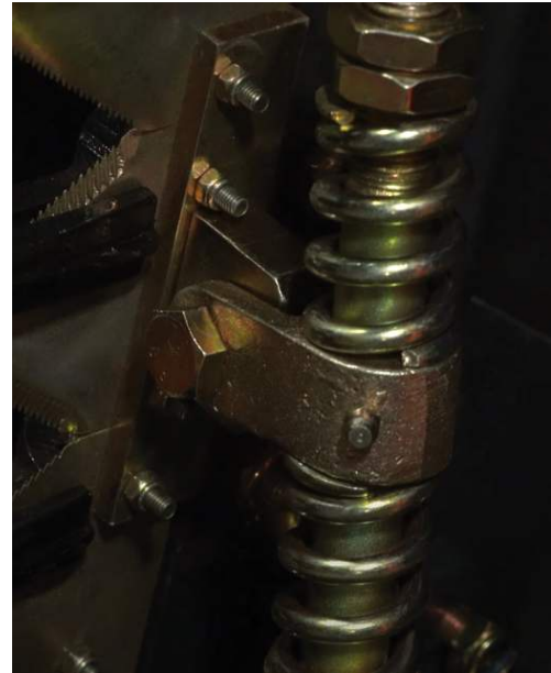
Connector Bracket on the sickle bar
