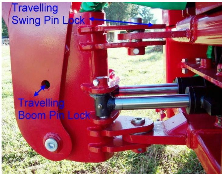
When transporting or dismounting backhoe, you must lock the backhoe's swing and boom. Position boom straight back and then slide pin through holes in boom & swing frame.
