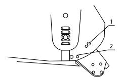
When adjusting the working height, loosen screw (1), remove screw (2) on both sides; The roller height (see following drawing); bolt the parts on the set position. The lowest hole is the highest working height; put the screw (2) into the set hole; tighten screw (1) and screw (2).
