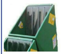
The upper chute on the chipper/shredder is for Leaves and twigs only. Do not use the funnel for vines or long branches such as Weeping Willows as they may clog the flails.
