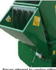
The lower chute is for longer and/or thicker pieces of yard waste. Depending on your model, you may cut up to a 3" x 5" in piece of wood.
