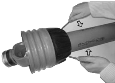
Prise Clasps Open to Release the Shield
