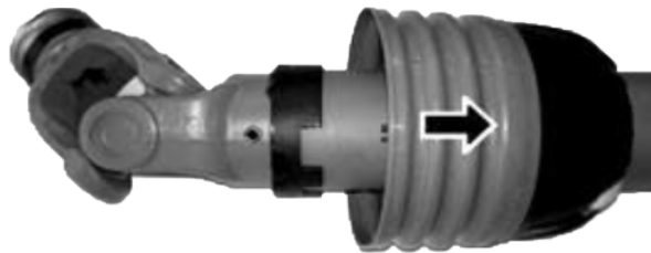
Slide Shield Back to Reveal Universal Joint
