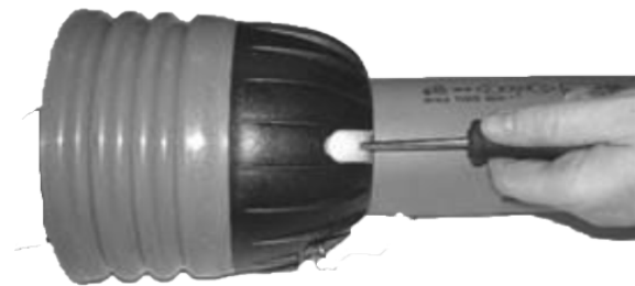
Insert Screwdrivers Into the Clasps
