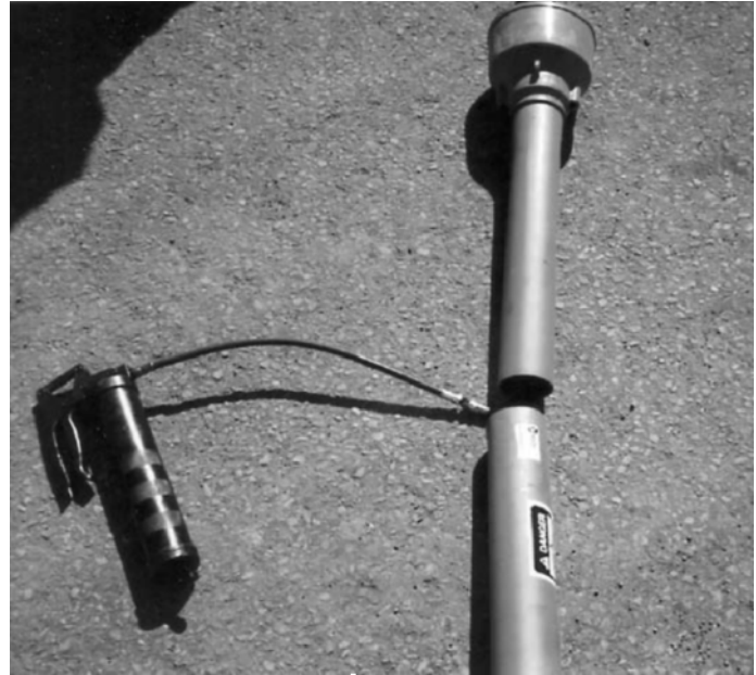
Fig. 31 PTO grease point
