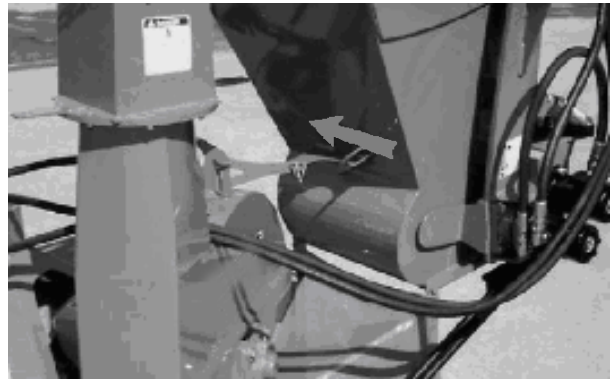
Fig. 5 HOPPER TRANSPORT LATCH
