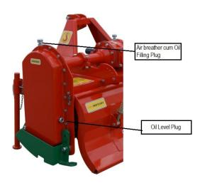
Check the oil level every 50 hours. Make sure it reaches the level plug on the transmission cover.
