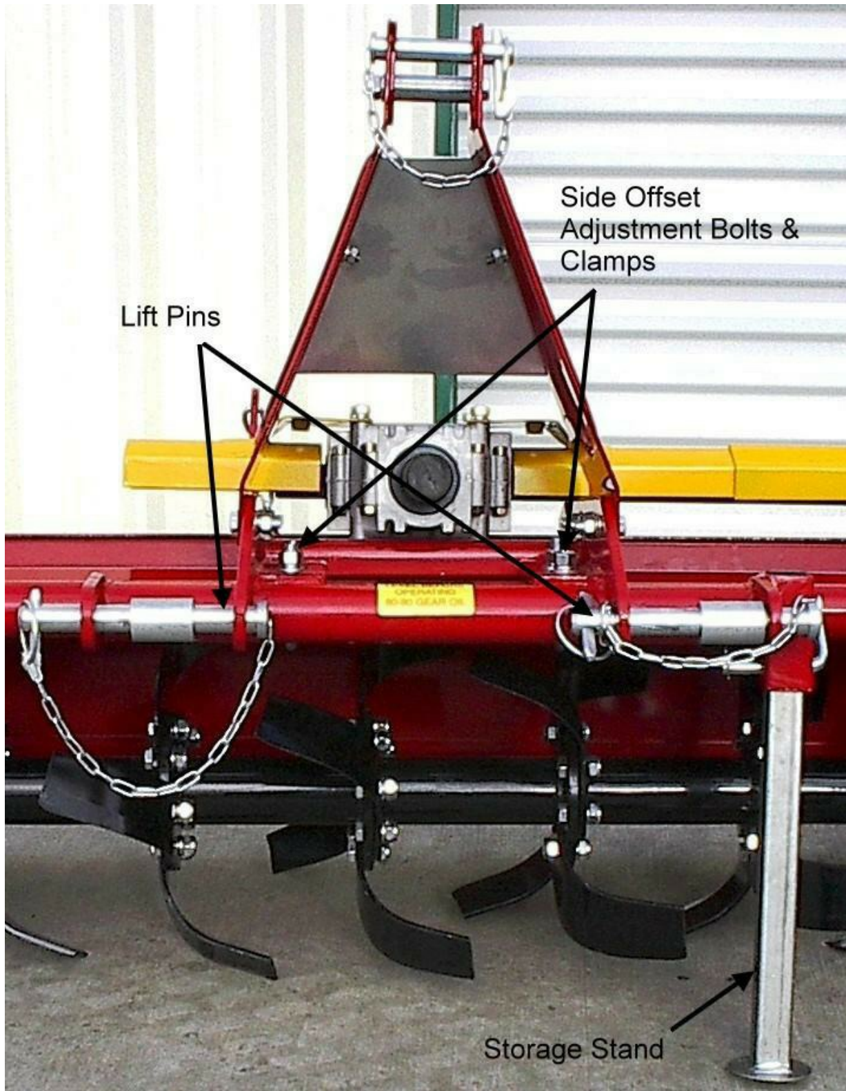
Offset Adjustment Bolts & Clamps, Lift Pins, and Removable Storage Stand
