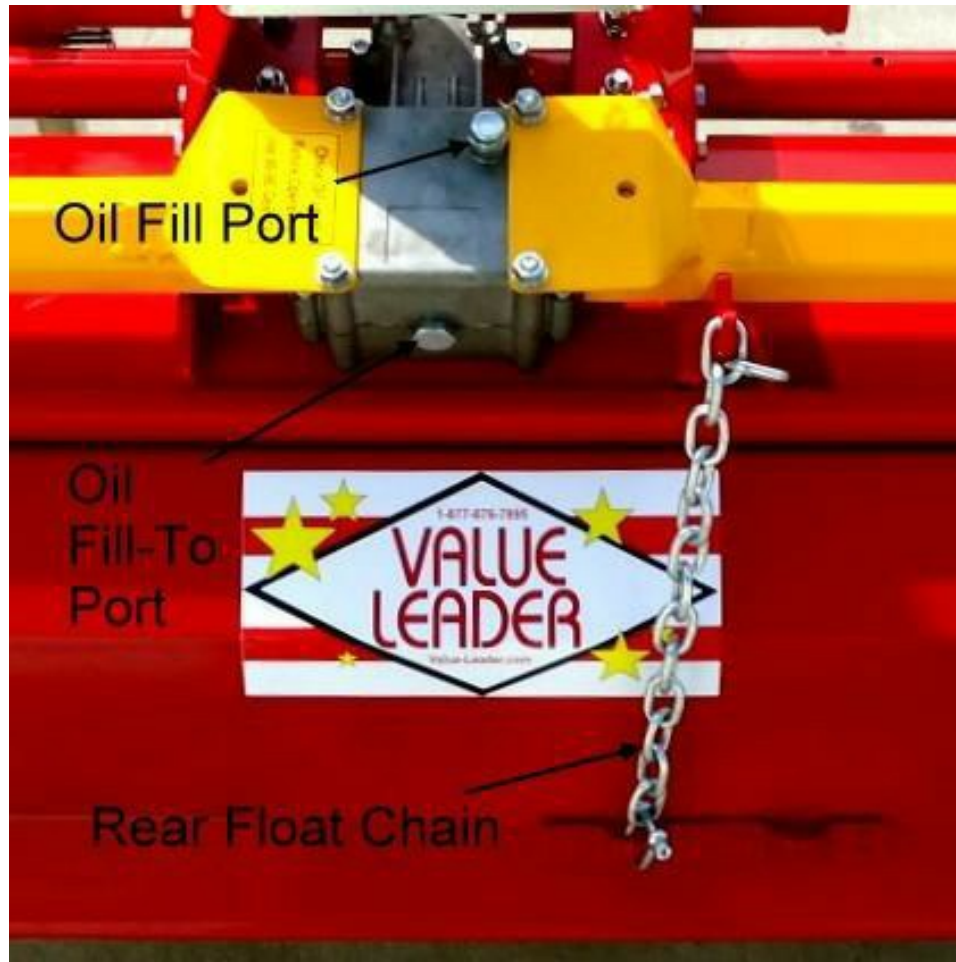
Gear Box Oil Ports & Rear Float Chain
