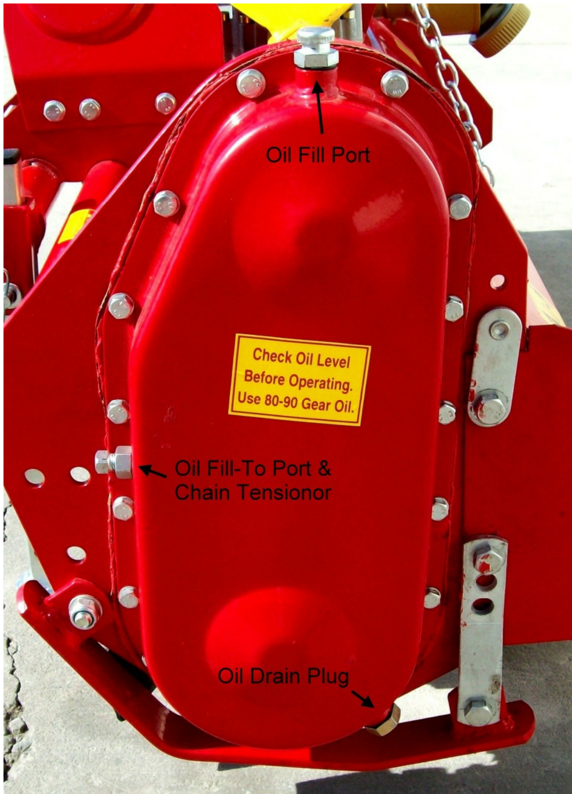
Chain Case Oil Ports & Tensionor
