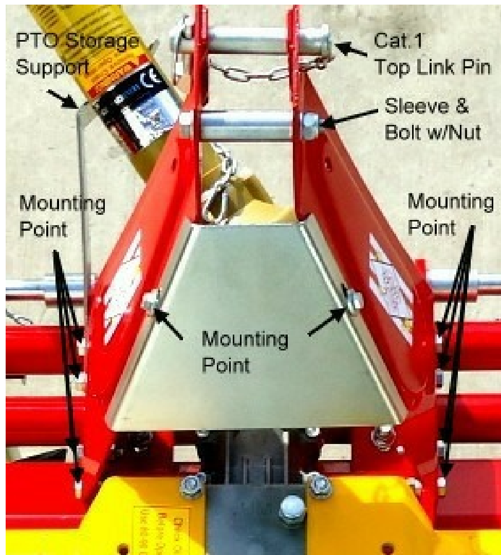
Mounting Plates, Top Link Pin, Sleeve & Bolt, PTO Storage Hook
