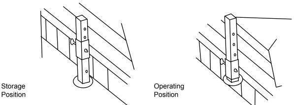
In order to keep the machine stable, lower the adjustment stand when the machine is stopped (see above drawing).
